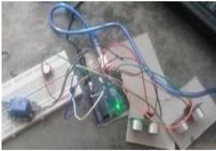
Gambar 8. Tampilan Sistem Dekat TV (Kontrol Jarak Nonton)
